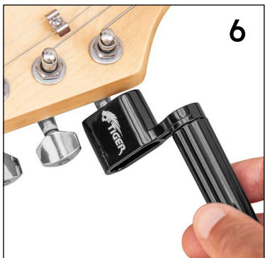
Wind the peg using a string winder, if you have one, until it is taut.
